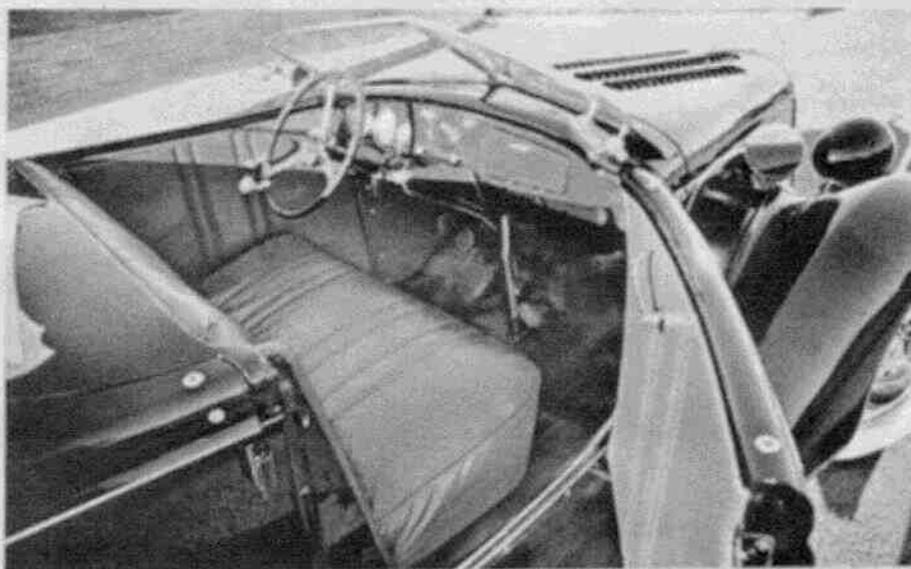
miniature masterpieces in themselves. Don Bridgman constructed the rear seat cowl by adapting the forward cowl section from a 1935 Ford roadster parts car. He then fabricated the supporting structure and magnificent surface panels blending it into the phaeton mid-section. Following this, Charles Proia took thirteen days to carefully hand-fit each of the windshields to the cowls.
