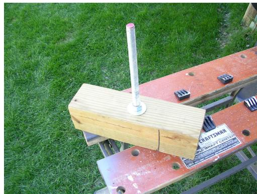
The base assembly would now clamp into the Workmate. The 8" wheel would rest on the hex nut, and the wheel rim and tire to would rest on top of that.
