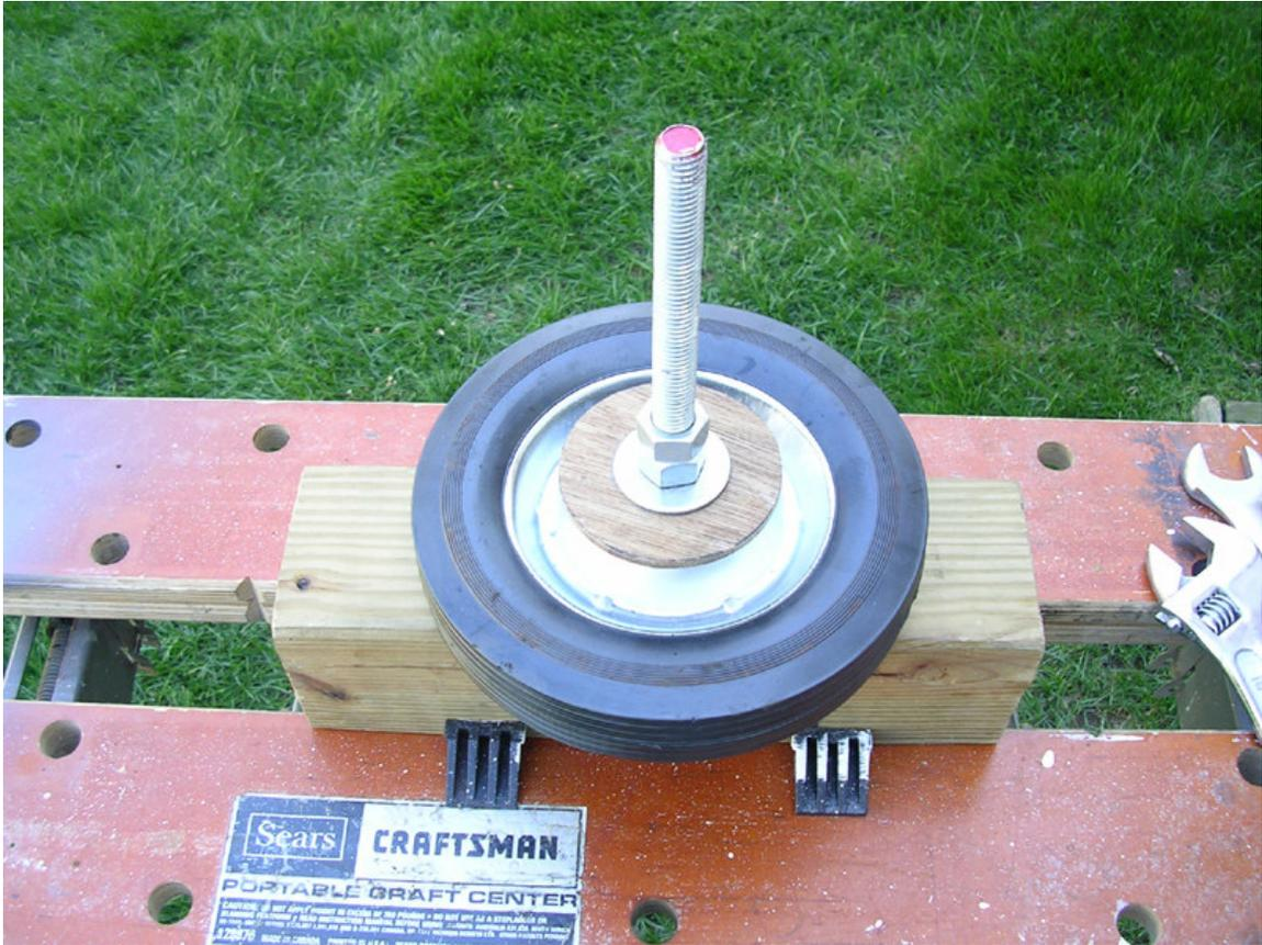
The original arm design was intended to hold a paint stripe wheel tool, and had adjusting stop nuts and wing nuts as shown in the picture. The outer block was two pieces, with a hole to mount and clamp the stripe tool. I decided that I would use brushes instead. A solid piece of wood could be used for the arm and hand rest with a 5/8" hole instead of the adjustable stops version.
