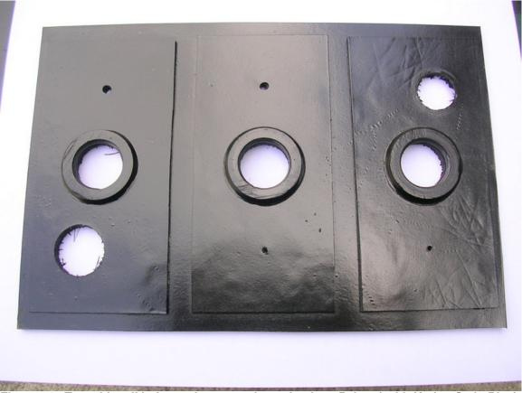
Figure 14 - Top with cell holes and cap openings glued on. Painted with Krylon Satin Black
