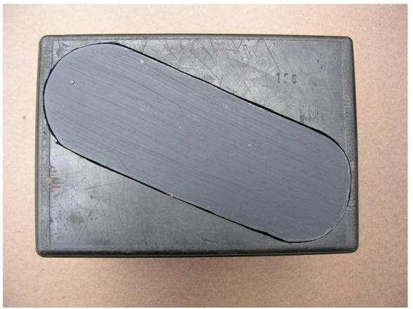
Figure 3 - Bottom of case with cutout and 3/4" base board mounted
