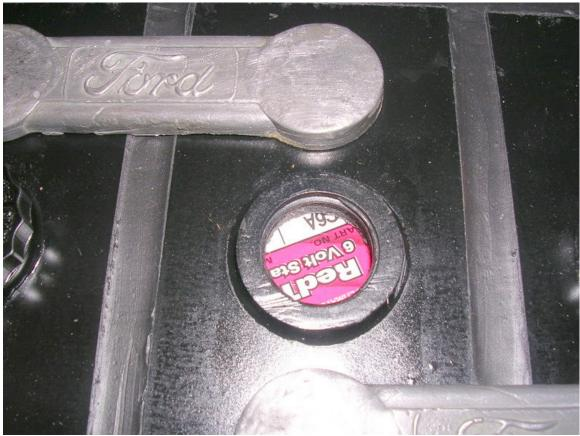
Figure 17 - Close up of cell top with battery cap removed
