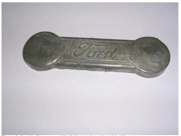
Figure 8 - Lead cell connector after being cut from the original battery.
