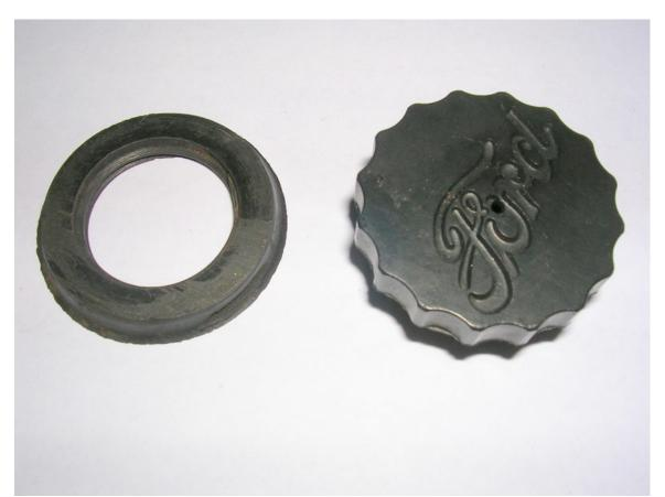
Figure 7 - Cap and cell top opening. The cell top opening was cut out and carefully ground down so that the radius is preserved. The cap will still screw in to the remaining thread portion.
