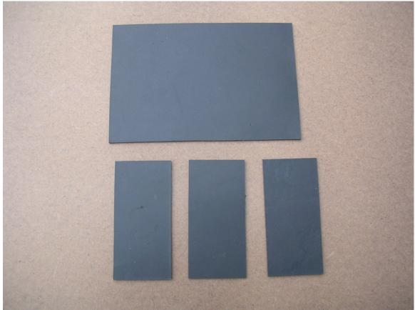
Figure 10 - Top and cell tops cut from mud flaps
